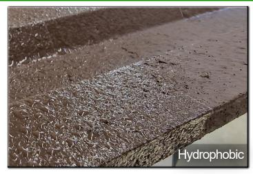
Note how the coated section of the tiles repel the water while the water absorbs in to the un-coated areas
